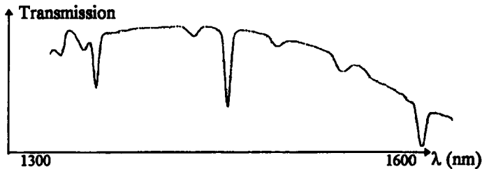
FIGURE 1 Transmission spectrum of a monomode fiber with a LPG.
